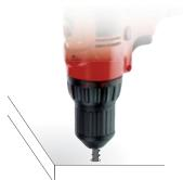
3 - Screw the assembly fitting into the face bored panel using a cross screwdriver.
