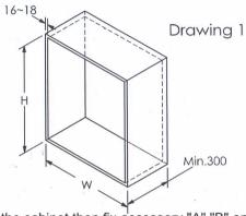
(2) Drill the side-board of the cabinet then fix accessory "A", "B" one by by one as the following drawings.
