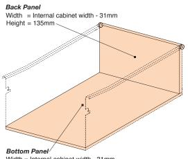
Width = Internal cabinet width - 31mm Length (Wooden back) = Drawer length - 2mm Length (Steel back) = Drawer length - 12mm
