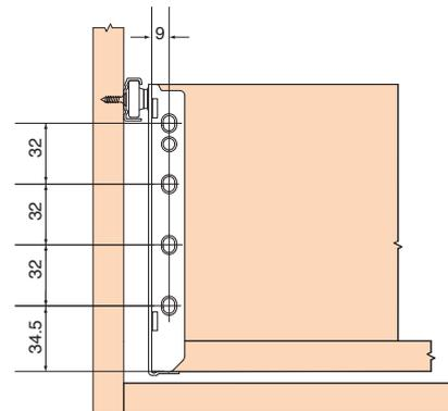
**Plug-In drilling dimension for bottom panel**
